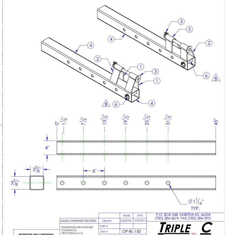
DIMENSIONS ARE IN INCHES TOLERANCES: FRACTIONAL±1/16 ANGULAR: MACH±1 BEND ±
